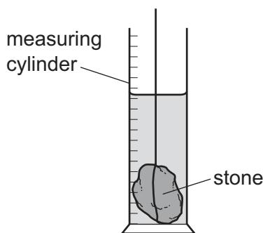
Which other apparatus does the student need to calculate the density of the irregularly shaped stone?
