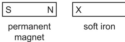
What is the induced polarity of end X of the soft iron and in which direction does the magnetic force act on the soft iron?
